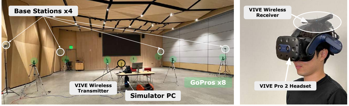
Figure 2.5: Left: The VR system set up in the classroom data collection space. Right: A pedestrian subject wearing the VR headset.
