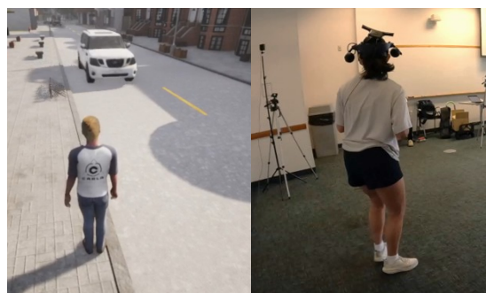
Figure 2.2: Example of JaywalkerVR simulation. Left: Subject's avatar in the JaywalkerVR from a third-person perspective. Right: Captured image of a subject wearing the VR headset in the data collection environment in the real world.
